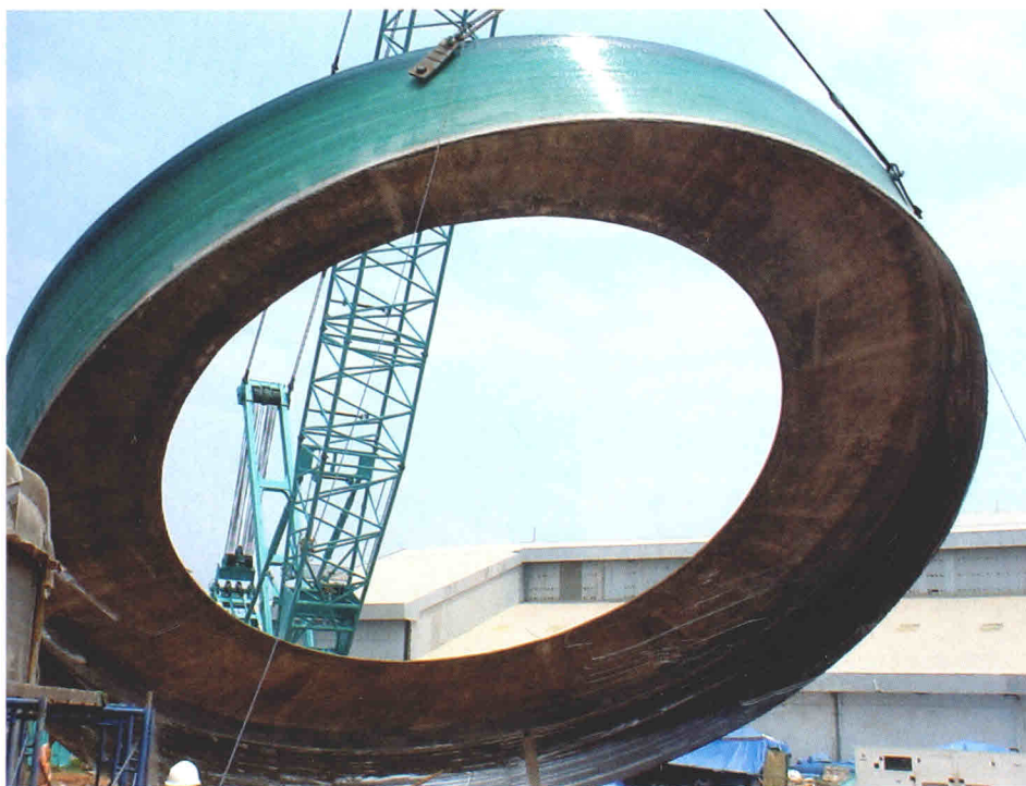
Tank knuckle being rotated for winding.
